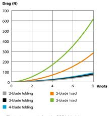
The test was carried out by SSPA Maritime Consulting. All propellers were mounted on a Saildrive propulsion system.
